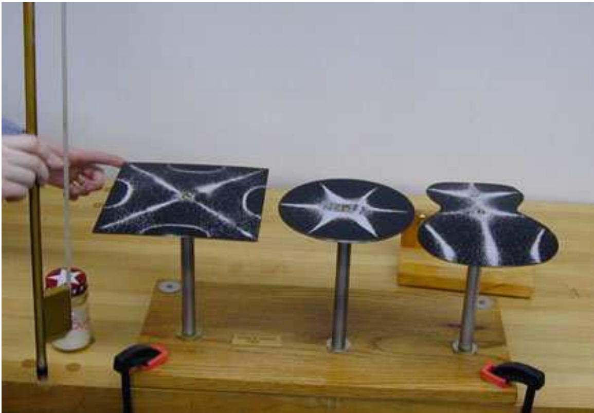
Figure 9. Chladni figures produced by bowing a steel plate while damping the plate with a touch of a finger. The patterns of standing waves are revealed by a sprinkling of salt that settles along the nodes where the vibration is minimal. Three plates are shown, one square, one circular, and a third shaped like the body of a guitar.
